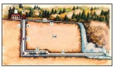
Visit history! Snoqualmie Falls Generation Project was the world's first total underground power plant. The powerplant was tunneled into the rock about 270 feet below the top of the falls. Water is diverted from the top of the falls, down a vertical penstock to the turbine cavity, and exits at the base of the falls. The plant was originally constructed in 1898, and has a capacity of
