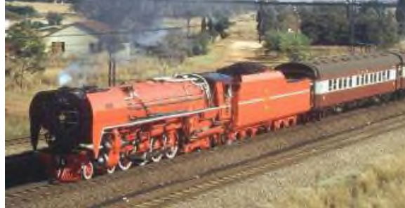
Locomotive #3450 with Porta modifications by David Wardale on test in South Africa, 1983
