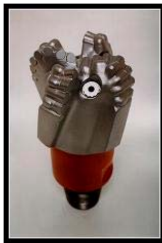
Figure 3 - Example PDC Drill Bit.
