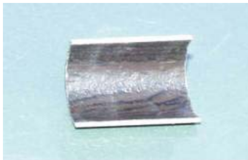
Figure 2. Typical Coated Coupon using Applied Modified Polyphenylene Sulfide (PPS) Coatings that result in PPS Coated Carbon Steel that Out-Performs Premium Alloys in Applications such as Heat Exchangers.
