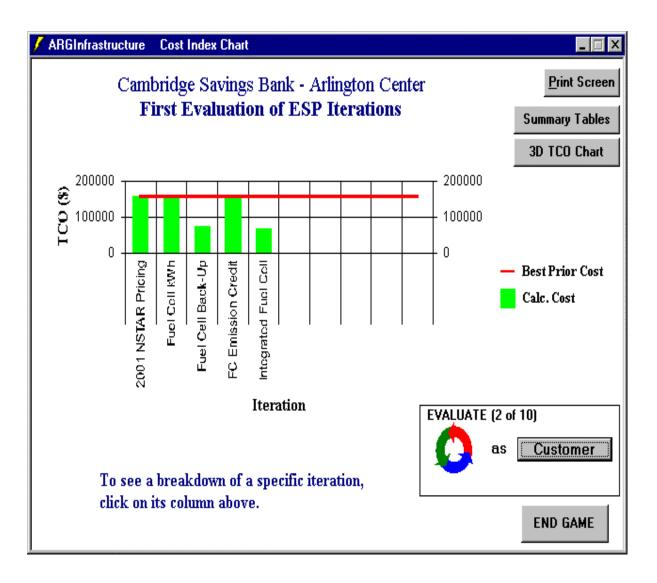
This screen is a snapshot of the *ARGIfrastructure* simulation representing the Total Cost of Operation benefit of applying a 5 kW PEM fuel cell to the critical IT and Telecom loads at a small bank in Cambridge Massachusetts. While savings and emissions are important and the latter when tallied with other projects will be substantial, the primary customer benefit results from avoiding damage at this bank.
