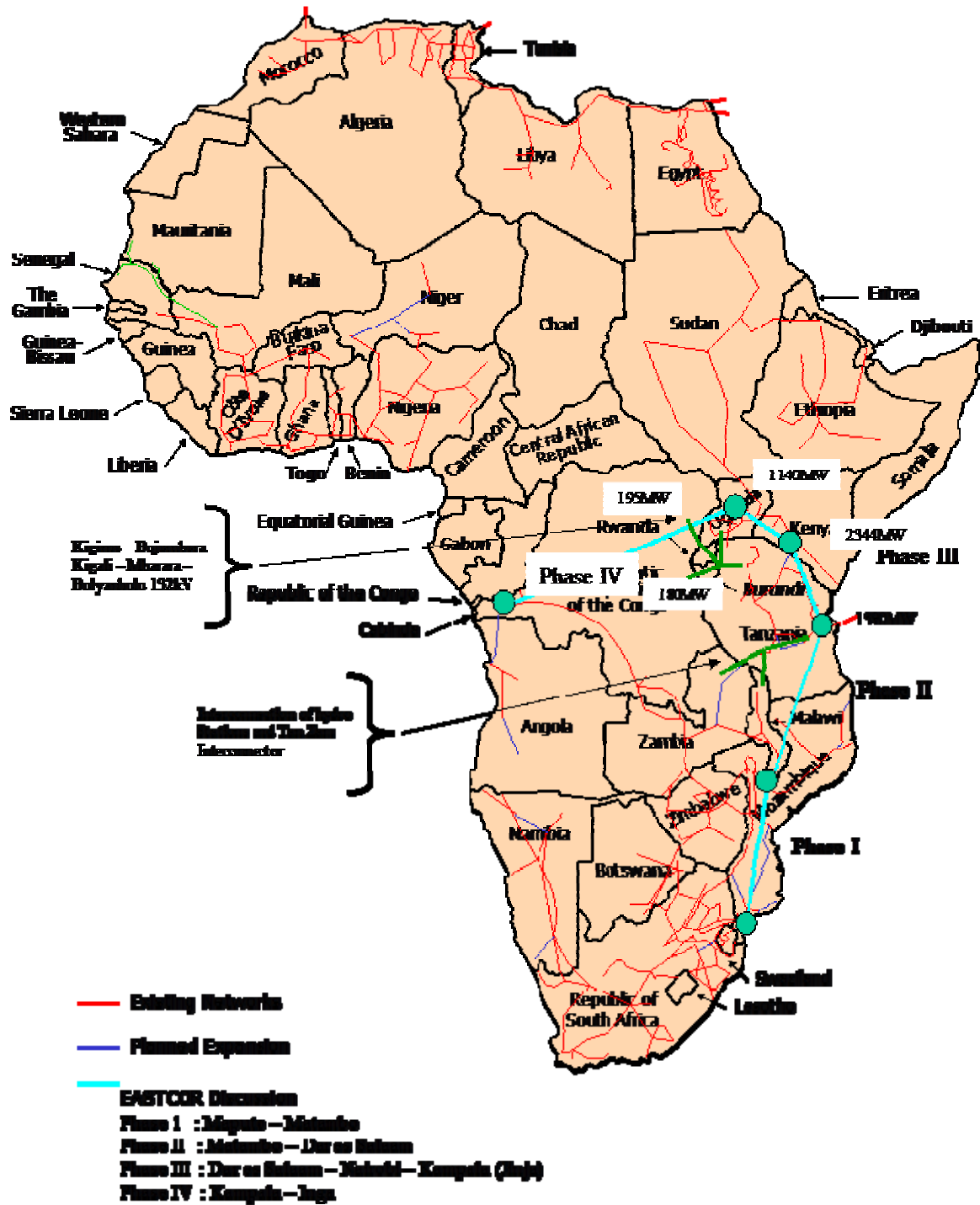
Fig. 1. The envisaged EASTCOR Inter-connector connecting loads and generation along the African East Coast
