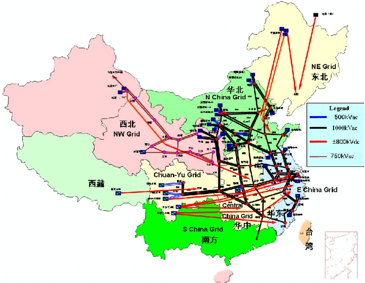
Figure 3 Interconnection of Chinese power grid in 2020 (planned)
