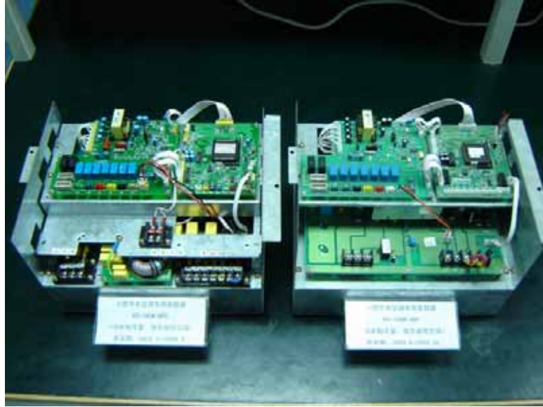
Figure 5 A prototype of frequency-converter for central air-conditioning developed by the Shenzhen RI
