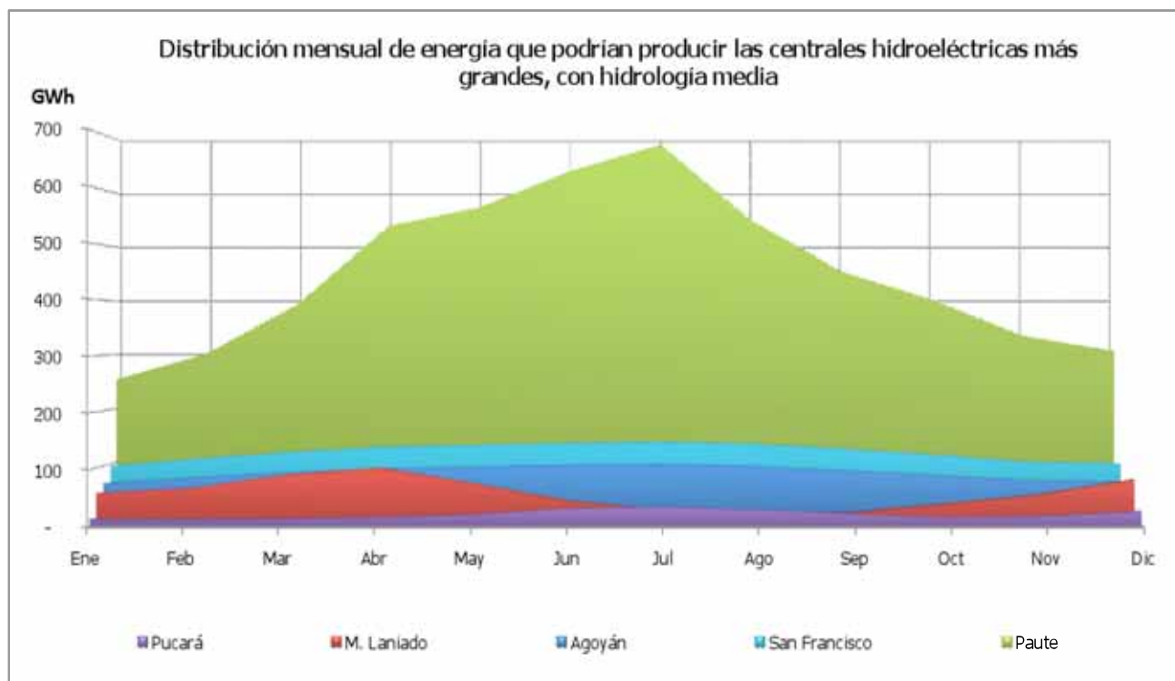
Figure 4. Generation of hydroelectric energy in medium hydrology
