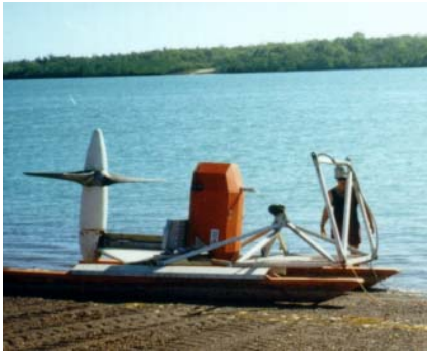
Figure5 The NTU – NT PAWA Kinetic tidal energy converter, on shore for maintenance
