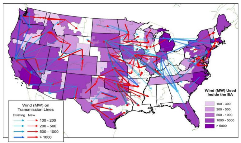
Total Between Balancing Areas Transfer >= 100 MW (all power classes, land-based and offshore) in 2030.
