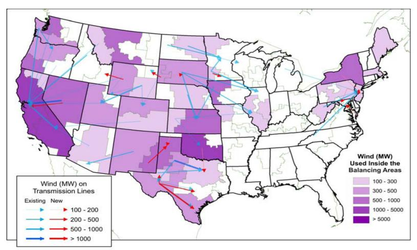
Total Between Balancing Areas Transfer >= 100 MW (all power classes, land-based and offshore) in 2012.
