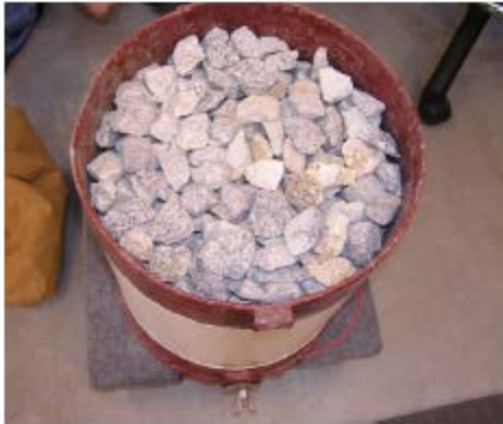
(c) Device Filled with #34 Washed Gravel
