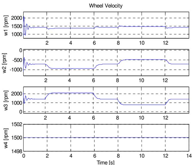
Figure 4 – Angular Velocity of the Reaction Wheels
