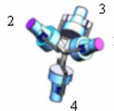
Figure 1 – Tetrahedron Configuration of Reaction Wheels
