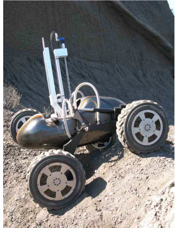
Fig. 1. The Scarab rover platform with passive rocker suspension.
