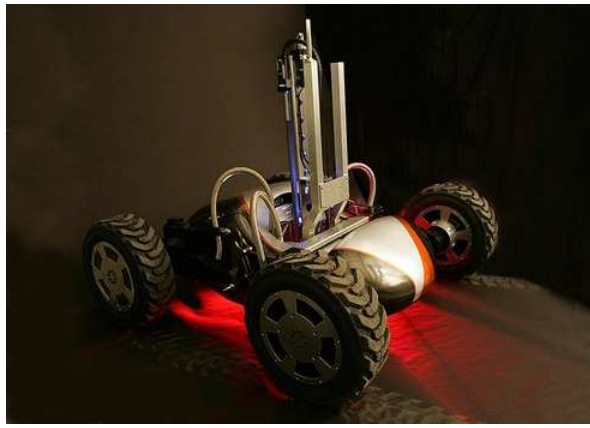
Fig. 2. The Scarab rover platform demonstrates optical-flow based visual odometry with active lighting for dark environments.
