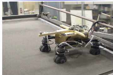
Fig.3: Experiments for the path following control with slip compensation on a loose side slope
