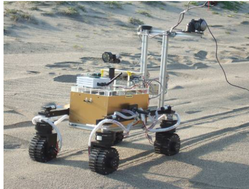
Fig.1: A rover test bed “El Dorado” in a beach sand environment
