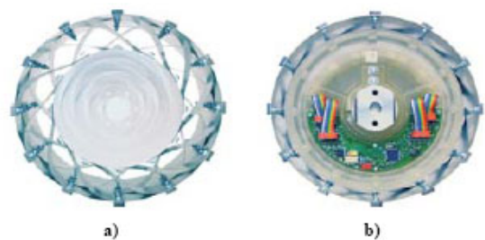
Fig. 11. iWheel12 flexible wheel a) Front view. b) Rear view with sensor rack.
