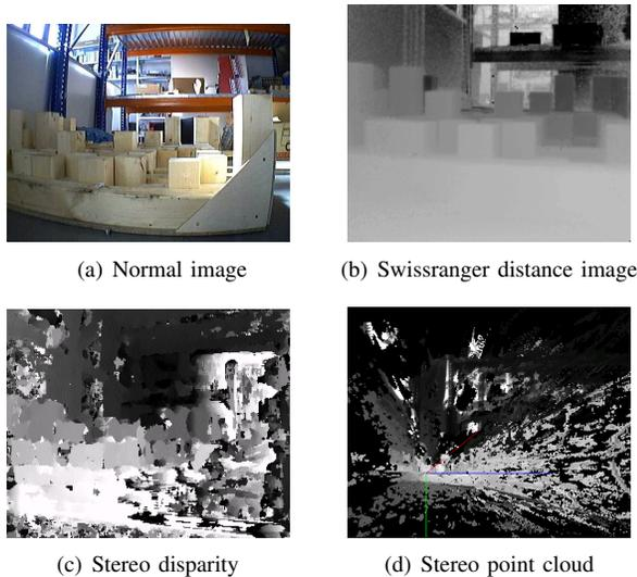
Fig. 4. Examples of sensor data.
