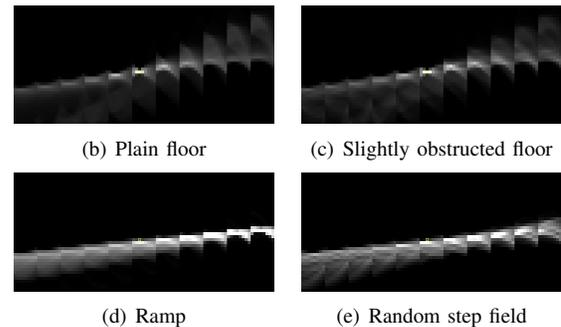
Fig. 5. Two-dimensional depictions of the three dimensional parameter space for several example snapshots. Distances are on the y-axis, where  $\rho_y$  iterates just once and  $\rho_x$  iterates repeatedly. Hits in the bins are represented by grayscale, the darker the less hits.
