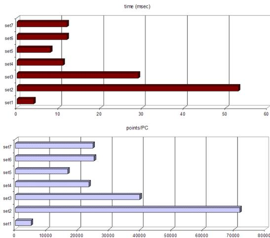
Fig. 7. The average time per classification directly depends on the average number of 3D points per snapshot in each dataset.
