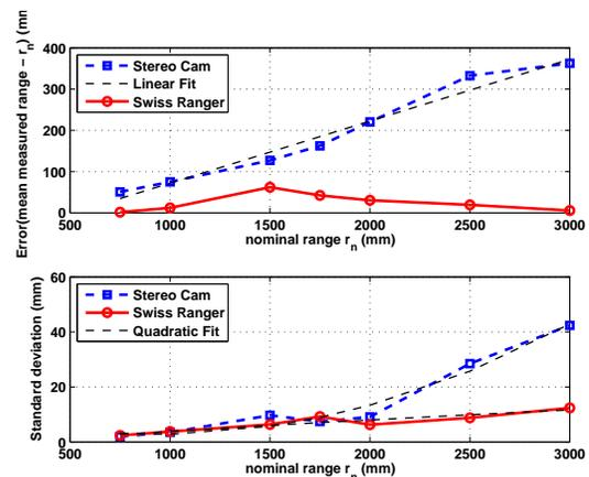
Fig. 6. Comparing the mean error and the standard deviation of the Swissranger versus the stereo camera. The standard deviation increases as the square of the range [21] for both sensors. The stereo camera is in general less accurate and also has a systematic error in the mean error which is linear with respect to the range.
