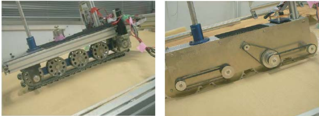
Fig.1: (left) “Mono-Crawler”, a single track test bed (right) an inline four-wheel test bed on the slope of dry “toyoura” sand
