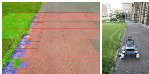
Fig. 5. An example of RTI prediction from remote appearance. The marks in the grass illustrate the influence on RTILE on the trajectory chosen by the rover.
