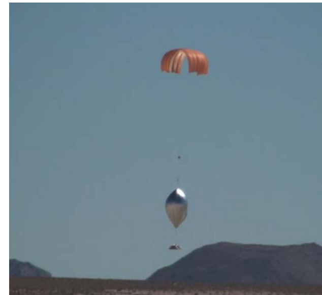
Prototype Venus balloon during aerial deployment and inflation test
