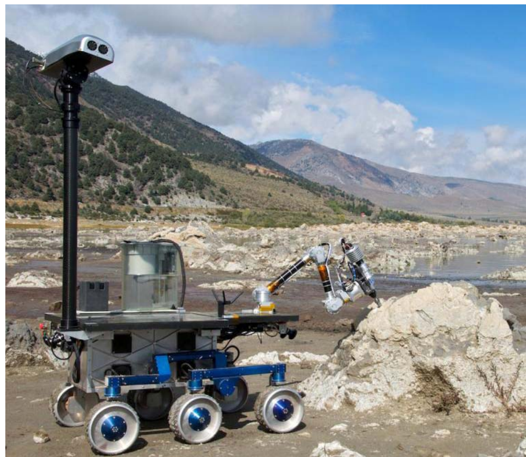
Coring Autonomy Field Test Mono Lake, CA – October, 2010
