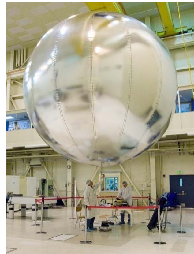
Prototype 5.5 m diameter Venus balloon
