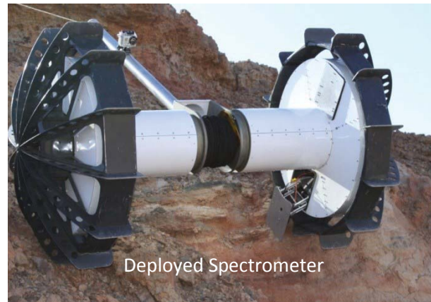
Figure 3. Axel deploying and acquiring infrared spectroscopic measurements and microscopic images from its instrument bay on exposed strata ( 40^\circ slope)
