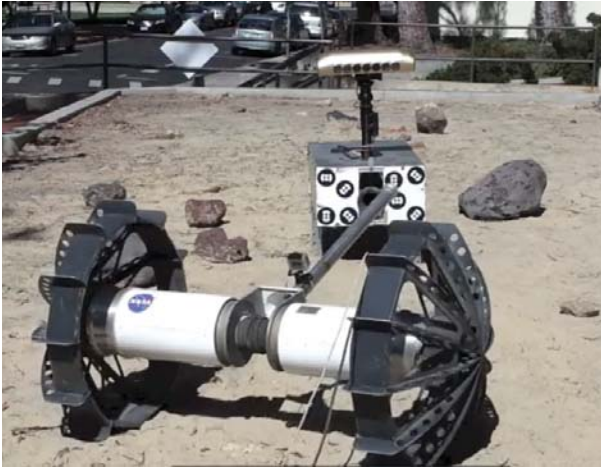
Figure 8. Autonomous vision-based tether-assisted docking of the Axel rover to the central module.
