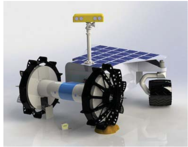
Figure 5. De-scope option of DuAxel with a single detachable Axel and fixed front steering wheels
