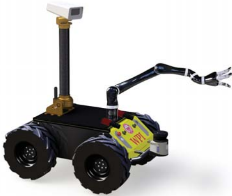
Fig. 1. CAD rendering of the Autonomous Exploration Rover showing the four-wheeled differential drive platform with 6-DOF manipulator, SICK LMS151 LIDAR, and stereo vision cameras.
