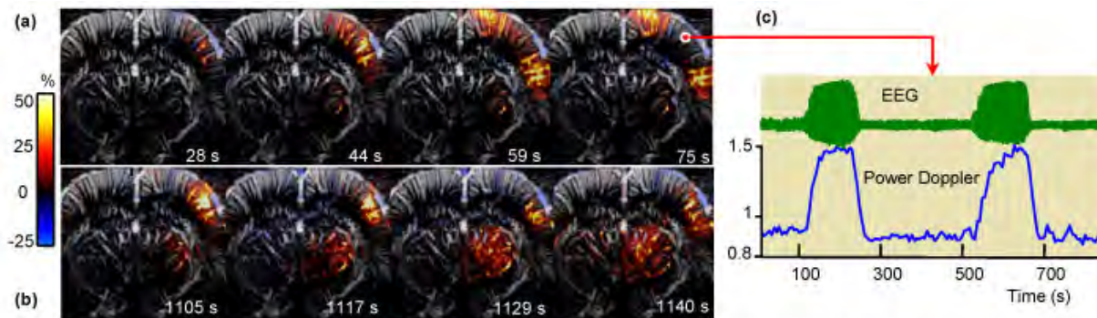
Figure. (a) and (b) Relative changes of Power Doppler superimposed on a control image at different times after seizure induction by 4AP injection. (c) Comparison between electrical activity (green) and Power Doppler signal (blue) at the same cortical location
