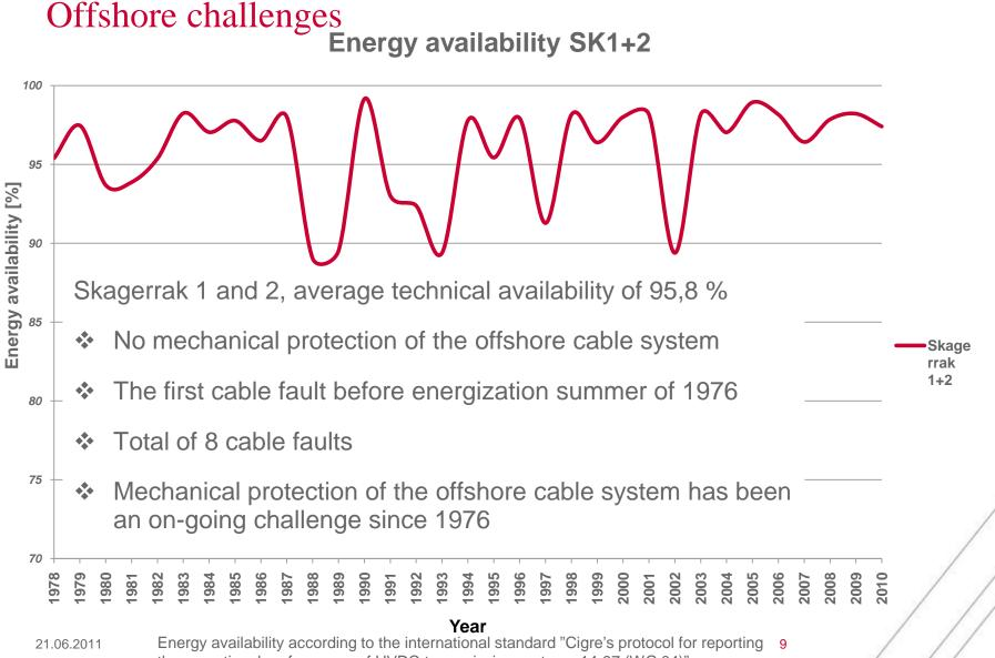
the operational performance of HVDC transmission systems 14-97 (WG 04)".
