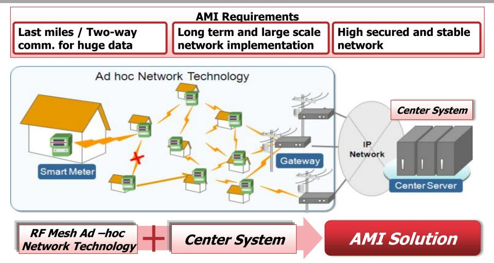
RF Mesh Ad-hoc NW & Cooperatively Binding Center System
