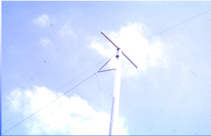
Horizontal Vee under broken conductor condition.
