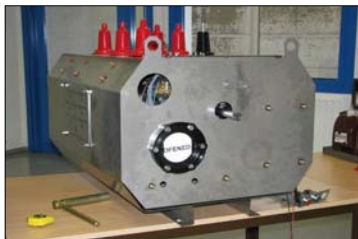
Medium voltage fast switch to transfer distribution load
