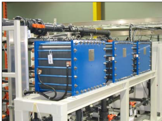
Cell stack assembly and piping – with pulse capability
