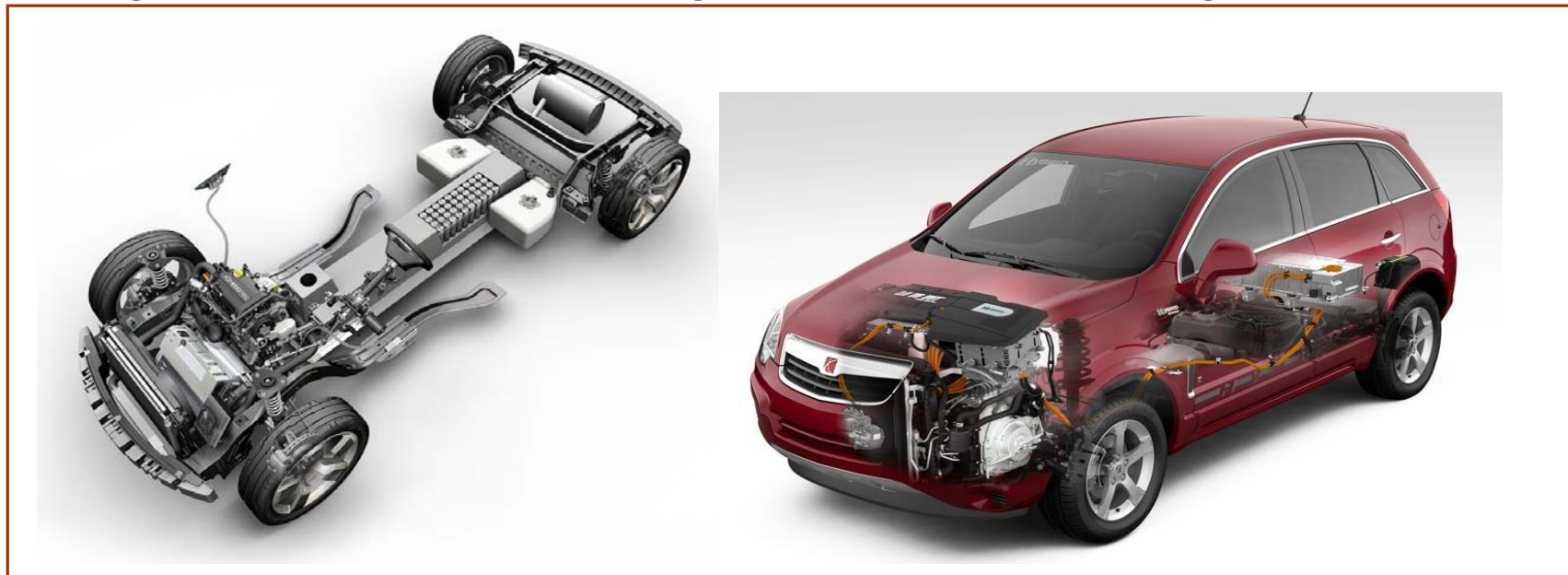
Range extended EV, series configuration.
