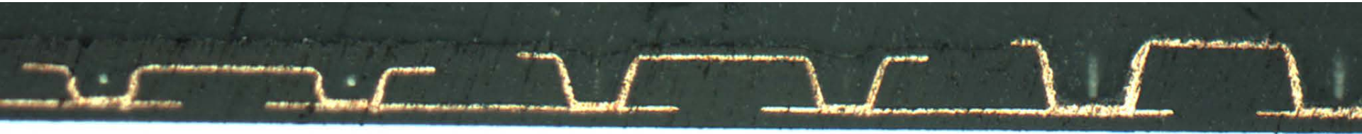
Laser drilled 3 Layers Standard diameter
