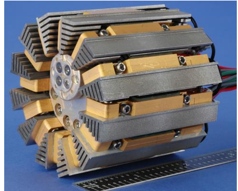
SSPA with the air-cooling fins attached. Mass of this unit is 0.47 kg and its dimensions are 2.4 inches dia x 2.5 inches.
