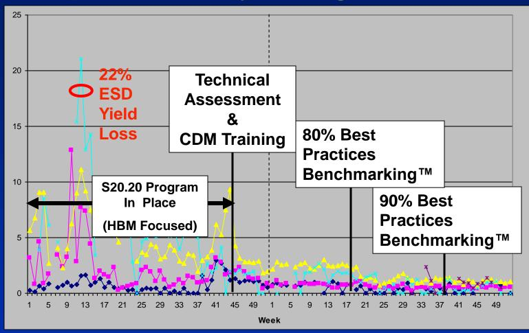
Note: Courtesy Herald Datanetics Itd. - 1<sup>st</sup> Class 0 Certified Manufacturing Operation http://www.dangelmayer.com/class-0-certification.php Each data point is confirmed ESD damage during production (typically 65 volt CDM/HBM ESD sensitivity) and different colors represent different products.
