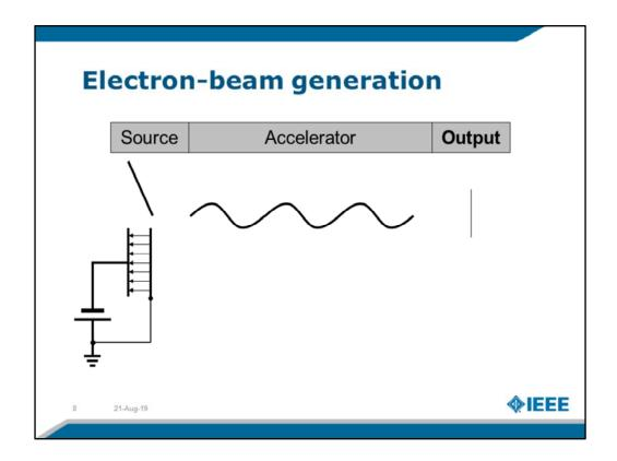
The electrons "surf" on the microwaves. If the electron bunches are phased properly with respect to the microwaves, then energy is transferred from the microwaves to the electrons.
