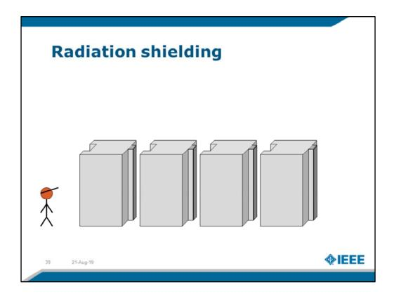
In practice, the shielding has a geometry to prevent a straight path that bypasses the shielding.
