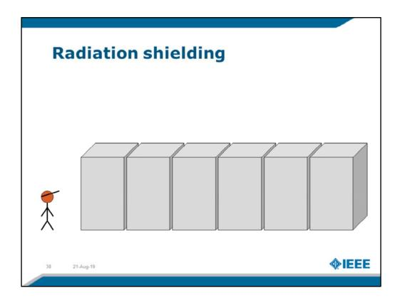
Shielding is roughly linearly proportional to electron energy, with some dependence on electron-beam current, with which the radiation levels outside the shielding are linear.
