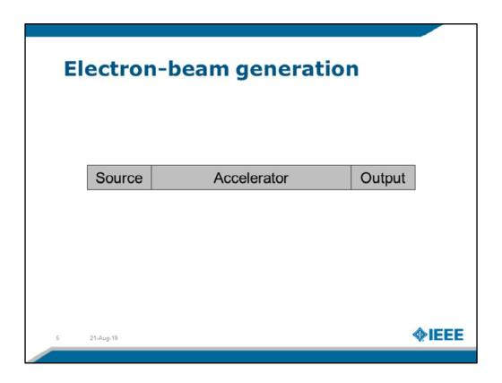
There are three parts to an electron-beam accelerator.
