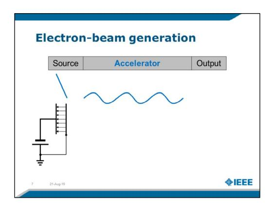
This electrical circuit is oversimplified. There is a third electrode, to draw off electrons from the emitting surface.
