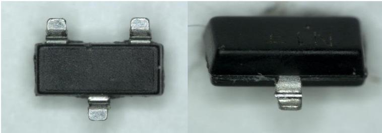
*Copper wire required wire bonding process changes resulting in parametric shifts and noise susceptibility that did not impact manufacturer's data sheet performance specifications. It DID effect legacy design performance as compared to devices with gold wire.*
