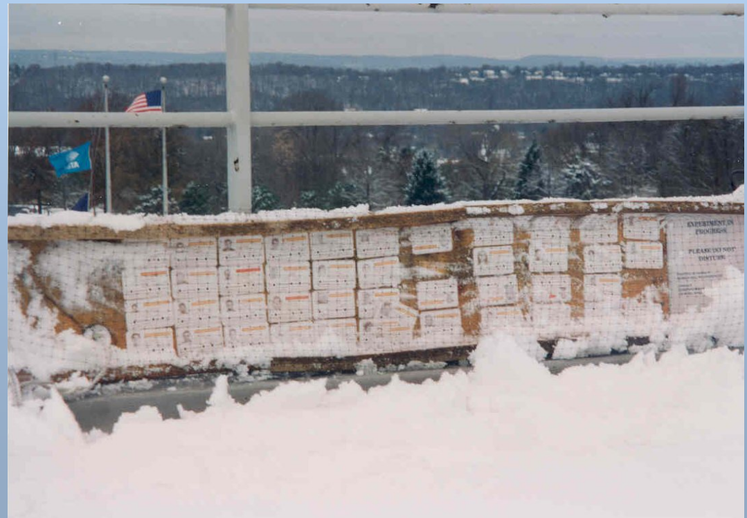
Card rack containing weathering cards on a snowy day.
