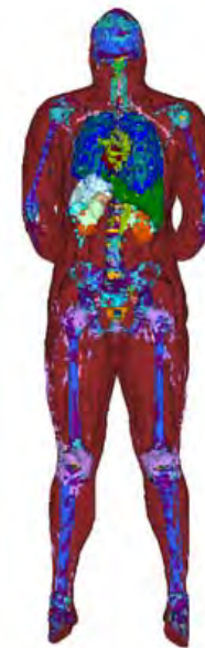
Radiation hazard analysis for personal radios carried inside an automobile. The human phantoms are modelled with the FEM, while the antennas and bodywork are modelled with the MoM.
