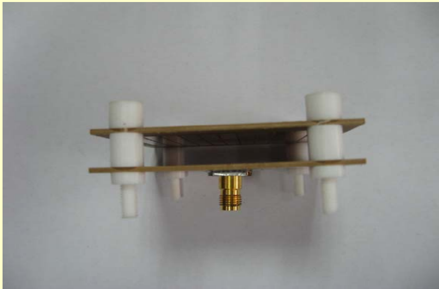
1-layer FSS Cover U-slotted patch Feed AMC-Base 11.7 mm ( 0.55 \lambda ) Height
