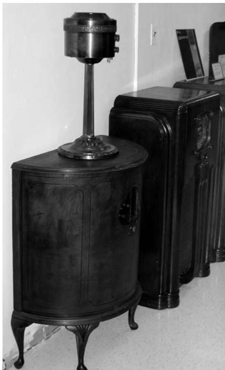
A 1930s remote-tuned radio. The object resting on the console is a remote tuner meant to be set on the floor away from the console. No matter to what station it was tuned, it put out a signal centered on 1 megahertz to the console.
