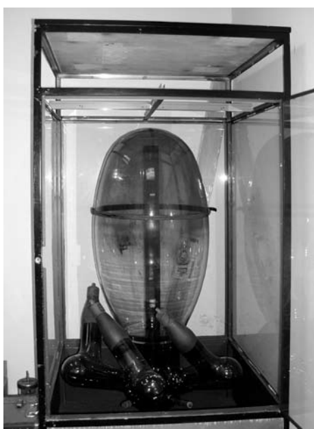
A 3-phase mercury vapor rectifier tube.
