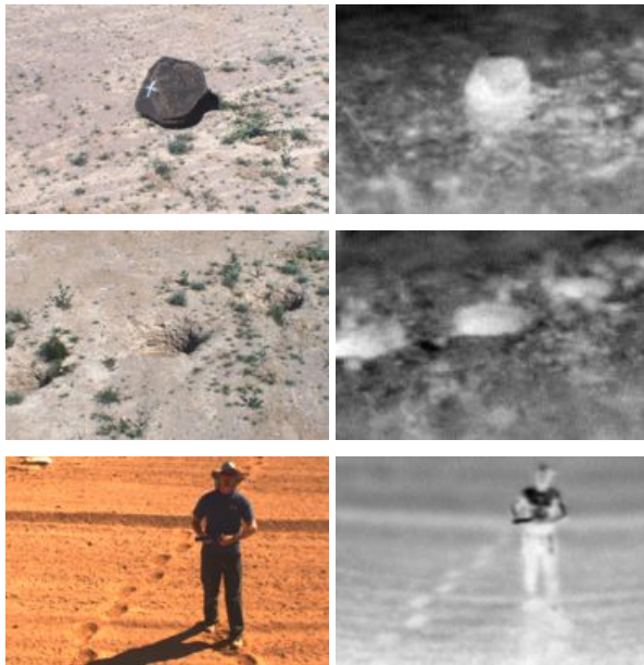
mmW and visible images of 2' boulder, 2' diameter holes, and person in Oasis LZ
