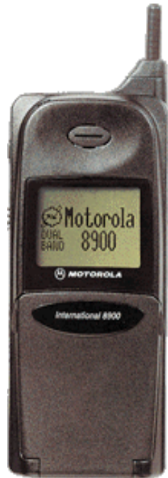
Motorola 8900 (1997) First dual band GSM phone 130 x 59 x 25 mm 248 g
