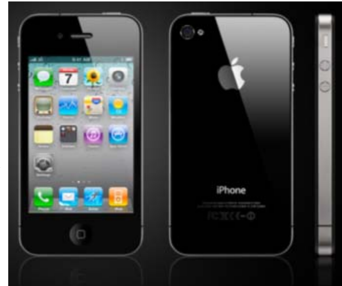
iPhone 4 (2010) 5-band GSM/UMTS + Bluetooth/Wi-Fi + GPS 115 x 59 x 9 mm 137 grams
