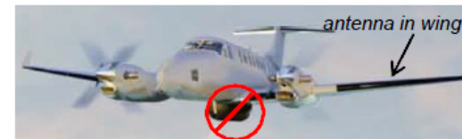
Airborne detection and surveillance systems require conformal antennas
