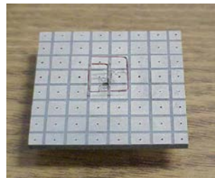
Zero-degree reflection phase for an antenna close to ground plane
