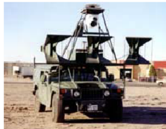
Forward looking ground penetrating radar systems require smaller antenna arrays
