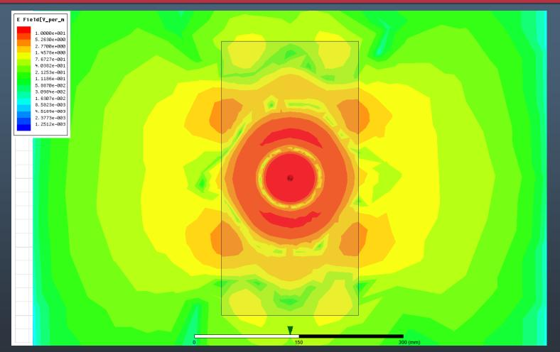
As one looks at the body from the top, concentric Electric Field rings become apparent and radiate out from the antenna source. Hot spots appear at various locations.
