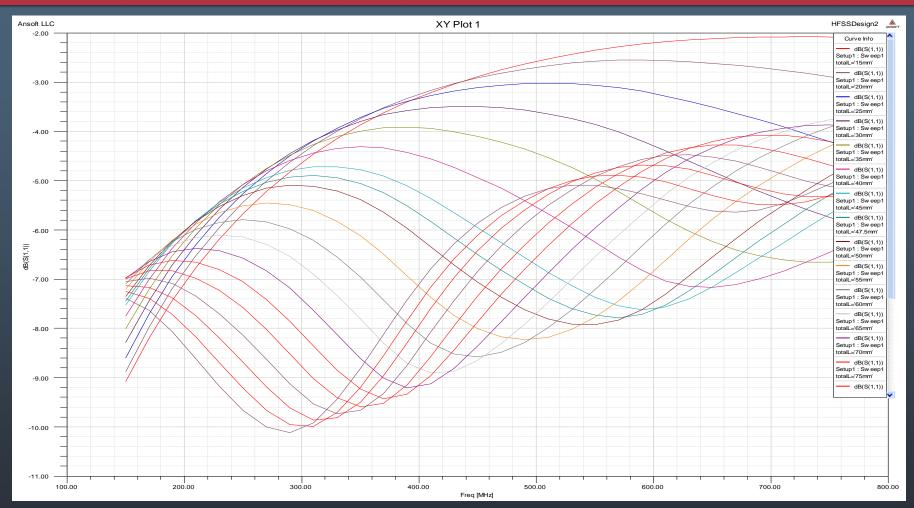
When  $\varepsilon_r = 50$ , the reflection coefficients for the parametric length study are shown above. These are slightly higher than in the case of  $\varepsilon_r = 40$  but show the same general behavior.
