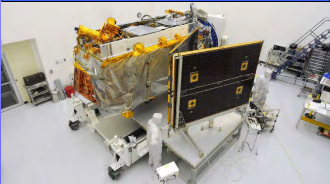
Solar Array Pop & Catch Pre/Post Dynamics & Post TVAC
