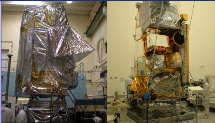
Solar Array Pop & Catch Pre/Post Dynamics & Post TVAC
