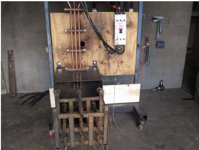
Arc chamber and calorimeter
