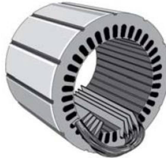
Stator Windings Partially Completed
