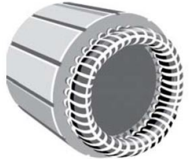
Stator Windings Completed
