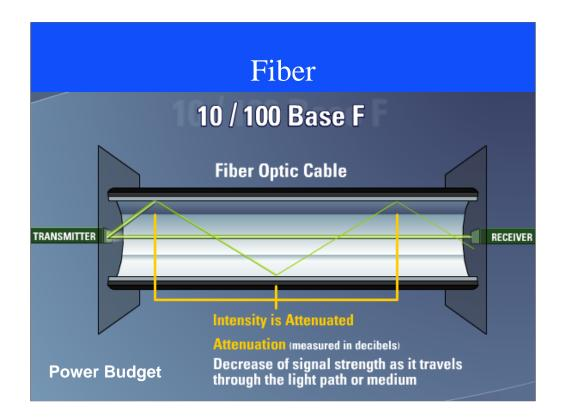
Power budget is the signal transmitter rated power minus the attenuation (cable, connections, splices, and cable aging) and the receiver's sensitivity
