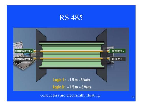
Up to 32 Devices, up to 4000 feet or 1200 meters, conductors are electrically floating which is why you can get the longer distances, only looking at difference so one may be at 100 V and the other at 106 volts, have a master and slaves
