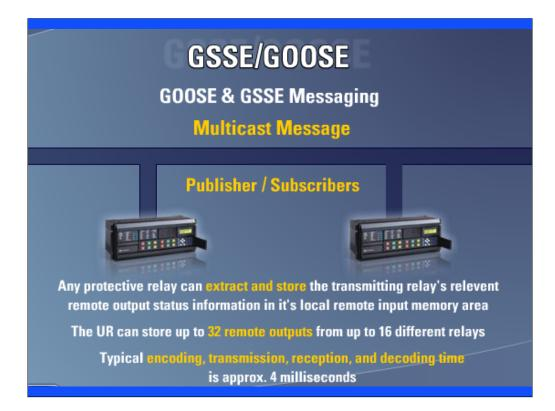
We have an example where we are sending a goose message from one relay to another relay that is 100 miles away and are making the second breaker trip within 8 ms.
