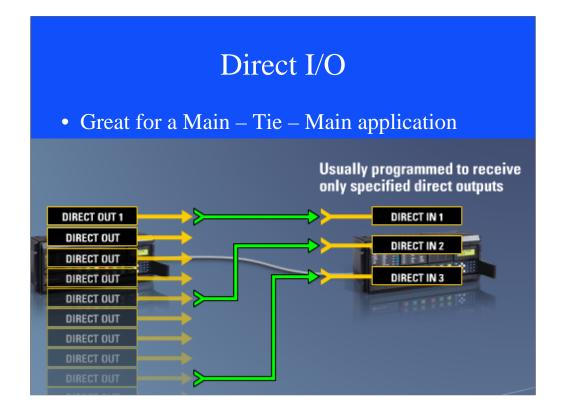
In the 750 relay you have to tie 11 of the 14 inputs to the other 2 relays. If one of the wires gets broken or miswired you probably will not know till it is too late. If the fiber get cut you will know in 8 msec or less. Can have redundant channels.
