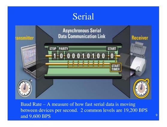
Asynchronous uses a start bit and a timer and measures the time to the center of each pulse. The Parity bit is used to check and make sure the data is correct and the stop bit is use to tell you the end of byte. You also have a Master and Slaves
