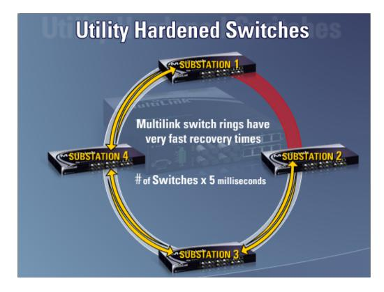
Has Normal and alternate port, managed and unmanaged, operating temperature of -40° C to +80° C
