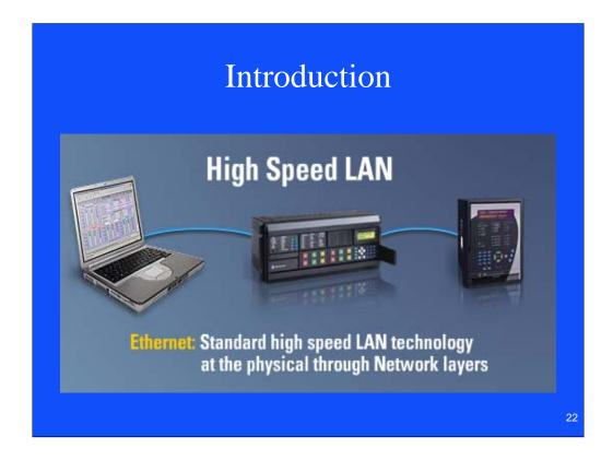
Relays are now available with Ethernet connectors and IP addresses built in.
