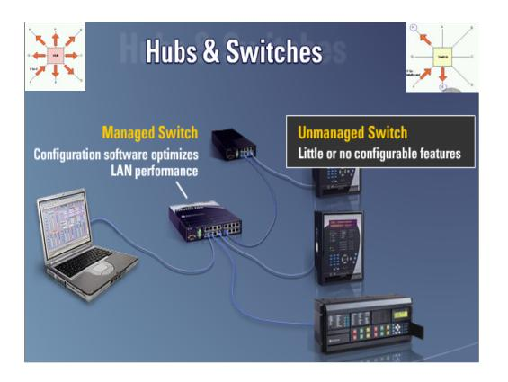
Switches can buffer the message so there are no collisions like a hub. Ours are Utility hardened, have output contact and dual power supply, can use on a ring topology.
