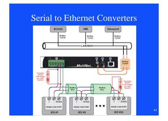
Converter may just change from serial to Ethernet or may also be a gateway and change from one protocol to another. You assign an IP address to the converter.
