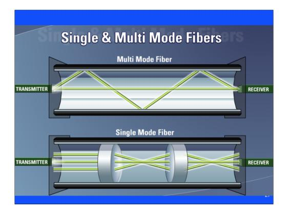
Multi mode has a shinny mirrored surface. Single mode keeps redirecting the light to the center, The center of multi mode is "doped" to slow down the signal so the reflected light gets there at the same time as what goes through the center.
