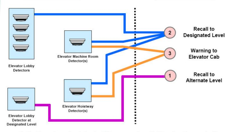
Activation of smoke detector(s) causes signal(s) to elevator controller
