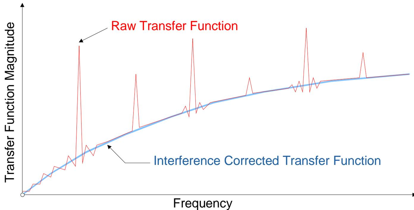
Correction Method: Based on quadratic rational transfer function fitting
