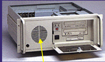
Shielding wall with opening for audio speaker
