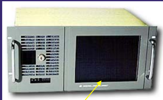
Opening for mounting display
