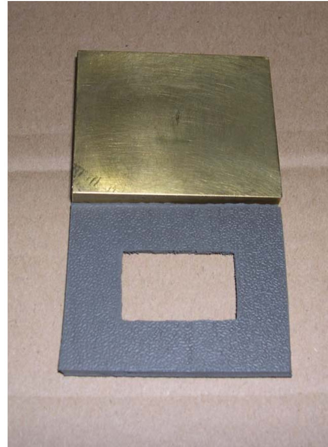
Fig2: HS baseplate w/500-mil thick material
