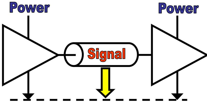
In a **SINGLE-ENDED** link there is a common (global) reference against which the signal is measured ("ground").
