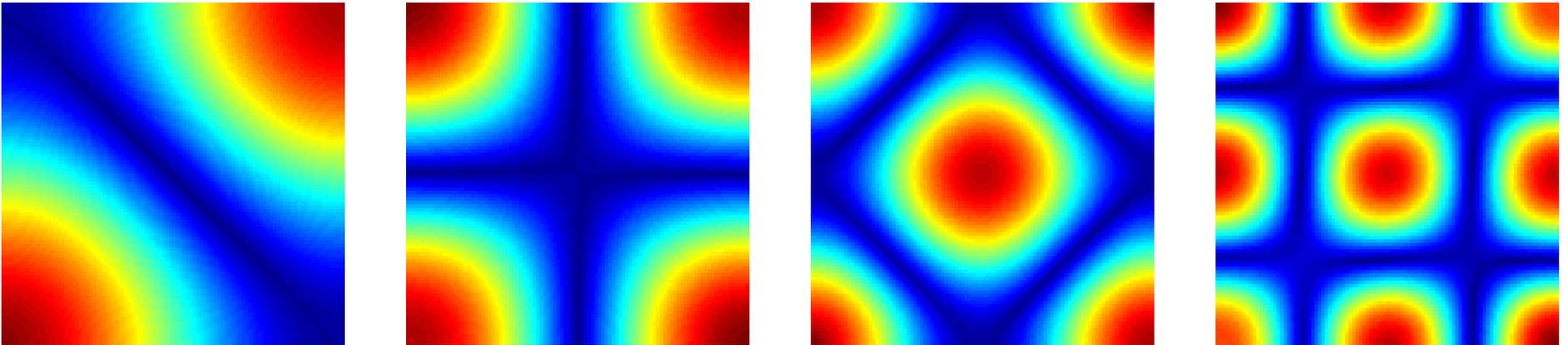
Examples of standing wave patterns on a rectangular power/ground plane pair.
