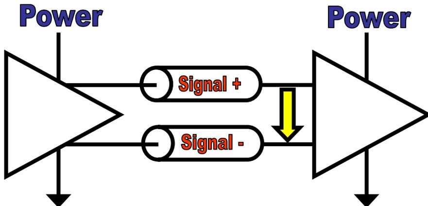
In a **DIFFERENTIAL** link the reference is the negative of the signal itself (which has to be transmitted as well).
