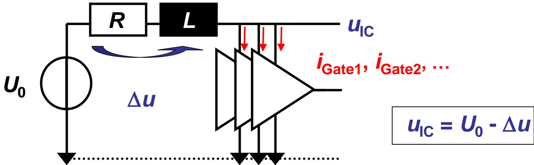
$$\Delta u(t) = \underbrace{R \cdot [i_{Gate1}(t) + i_{Gate1}(t) + \dots]}_{\text{"DC-drop or IR-drop"}} + \underbrace{L \cdot \frac{d}{dt} [i_{Gate1}(t) + i_{Gate1}(t) + \dots]}_{\text{"\Delta I-drop or \Delta I-noise"}}$$
