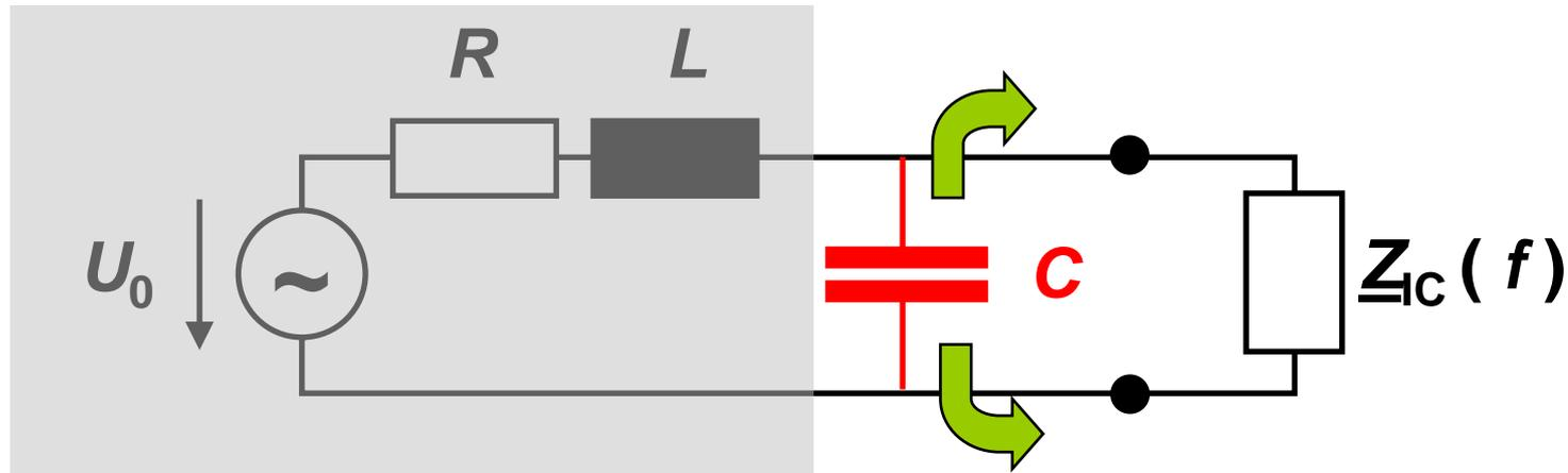
**Frequency domain:** Beyond the resonance frequency the capacitor decouples the part of the PDN that lies "left" of him, i.e. the IC sees only the impedance of the capacitor.
