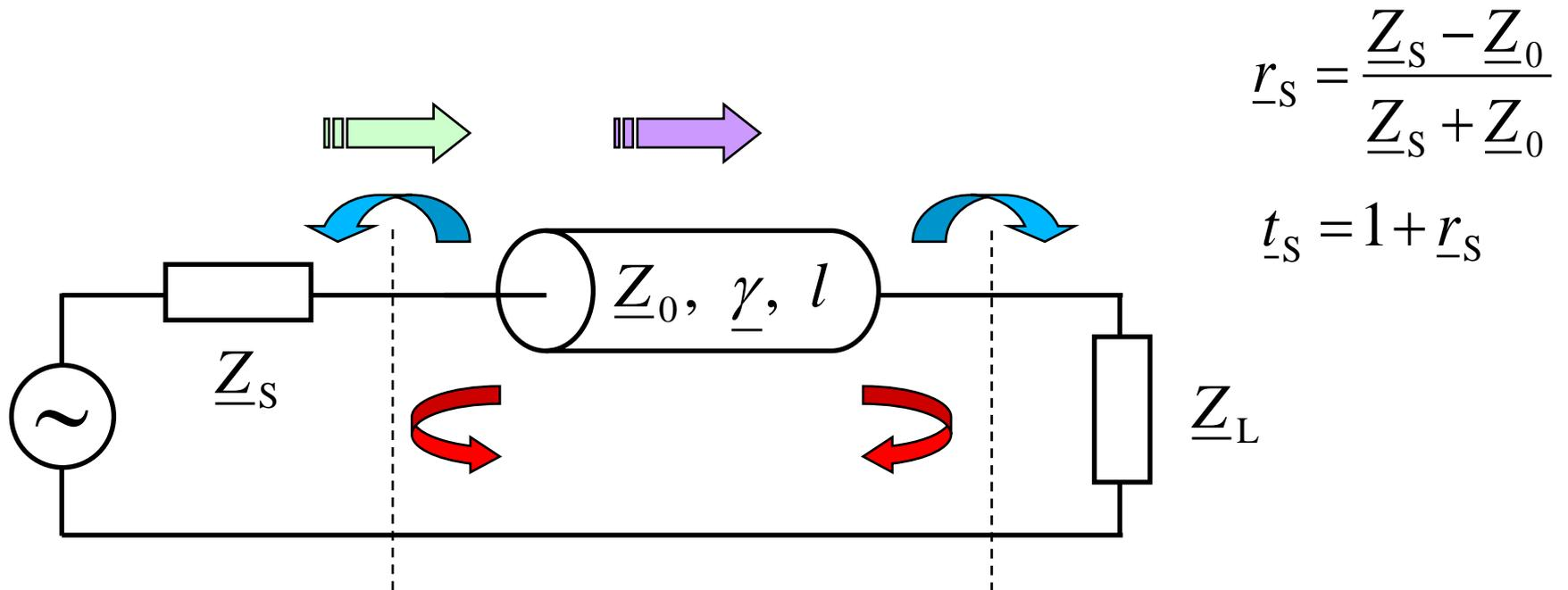
$$\underline{r}_S = \frac{\underline{Z}_S - \underline{Z}_0}{\underline{Z}_S + \underline{Z}_0}$$
