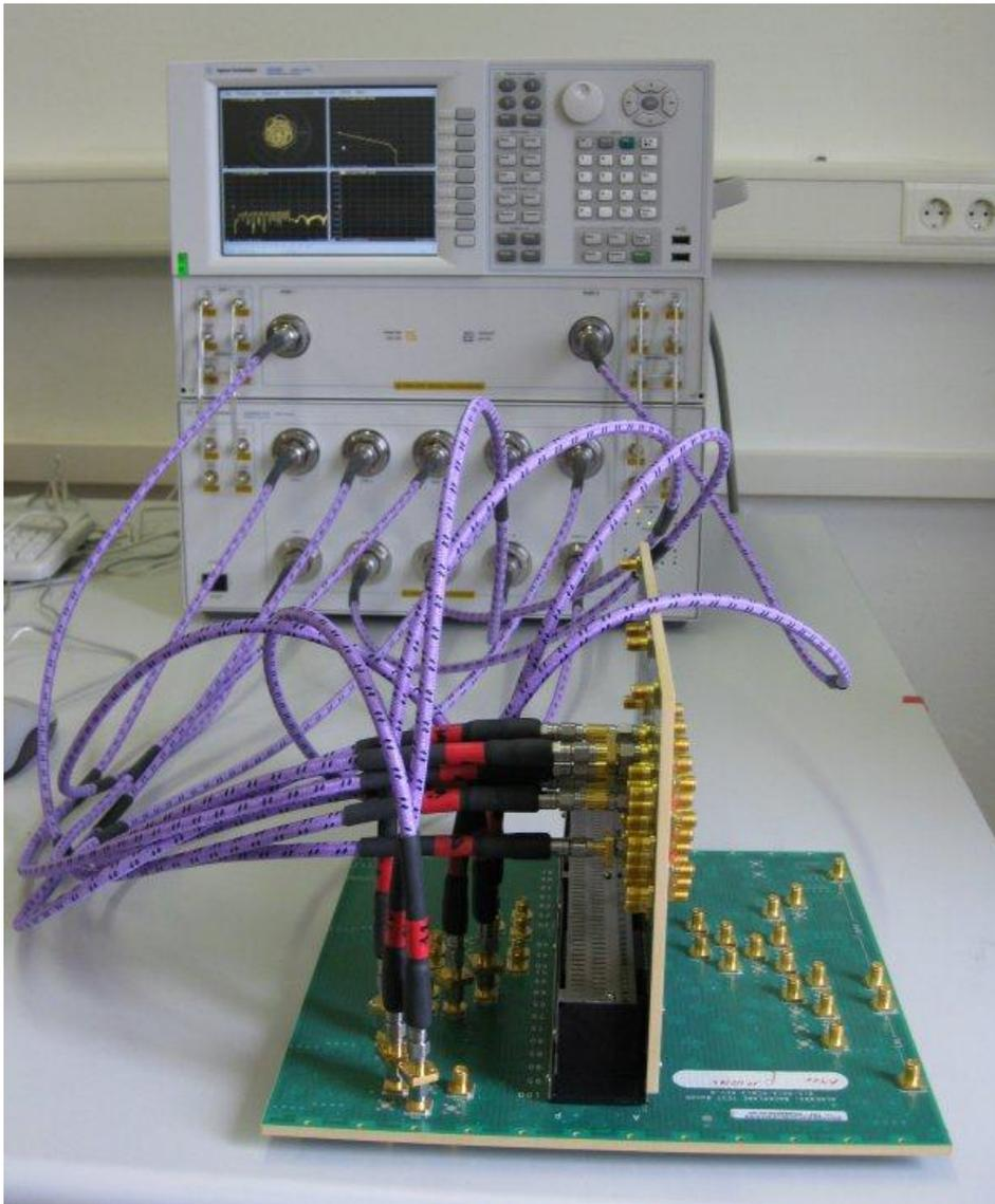
Agilent Vector Network Analyzer 8364C with 12-port extension at Institute of Electromagnetic Theory (TUHH)
