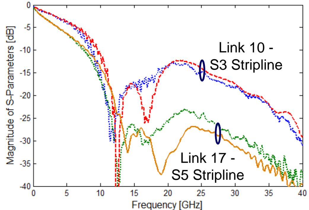
Models capture the salient features of the hardware response despite the drastic model simplification
