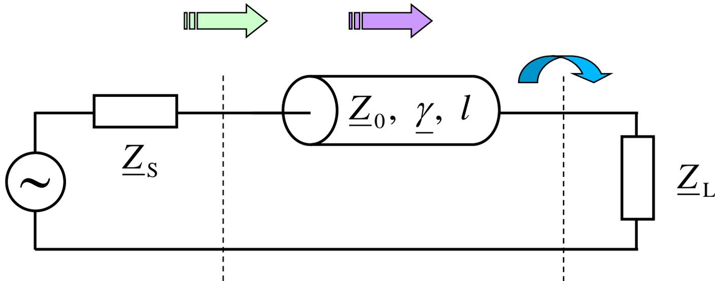
$$\underline{Z}_L = \underline{Z}_0 \rightarrow \frac{\underline{u}_2}{\underline{u}_0} = \underline{a} \cdot \underline{H}$$
