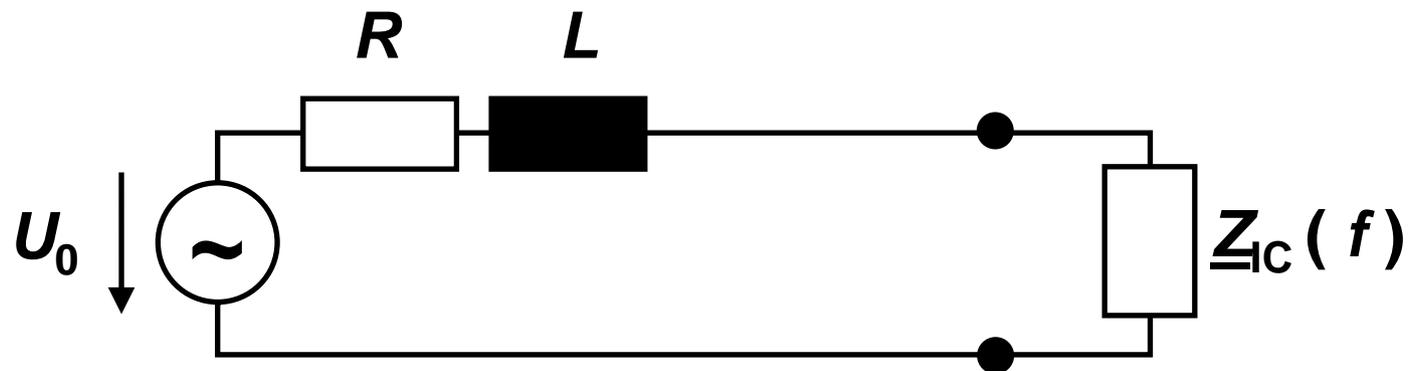
$$\begin{aligned} Z_{\text{PDN}} &= R + j\omega L \\ &\approx j\omega L \\ &\text{(for large } \omega) \end{aligned}$$
