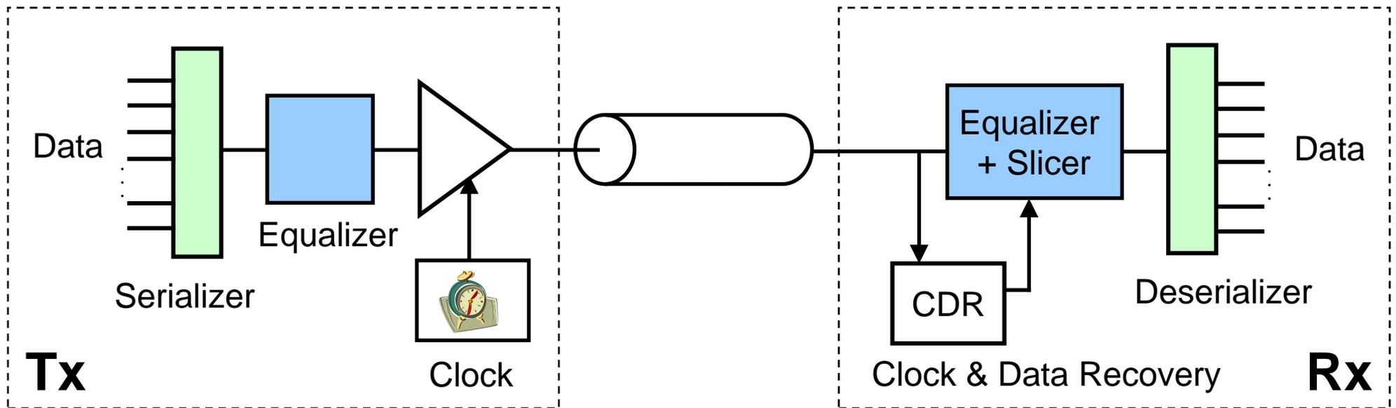
The technology is typically CMOS with the links being voltage mode, unidirectional, serial, point-to-point, and source-synchronous. For improved bandwidth equalization is typically used in the Tx, Rx, or both.
