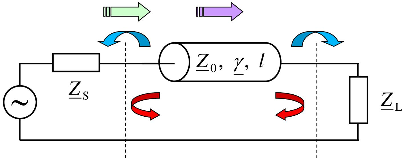
$$\Rightarrow \frac{\underline{u}_2}{\underline{u}_0} = \frac{\underline{a} \cdot \underline{H} \cdot \underline{t}_L}{1 - \underline{H}^2 \cdot \underline{r}_L \cdot \underline{r}_S} = ??$$
