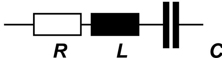
$R$  is also called the **EQUIVALENT SERIES RESISTANCE (ESR)** and  $L$  the **EQUIVALENT SERIES INDUCTANCE (ESL)**.
