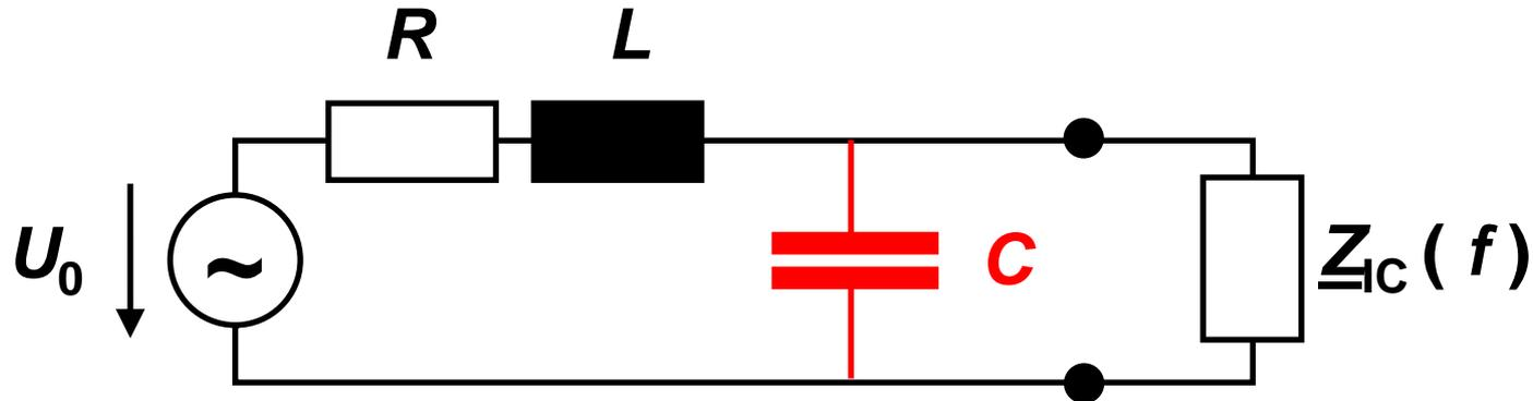
$$\underline{Z}_{\text{PDN}} = \frac{R + j\omega L}{1 + j\omega RC - \omega^2 LC}$$
