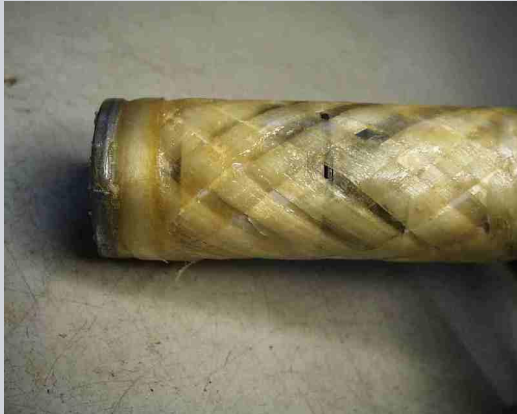
Fibre-glass wrapped around MOV resistor column
